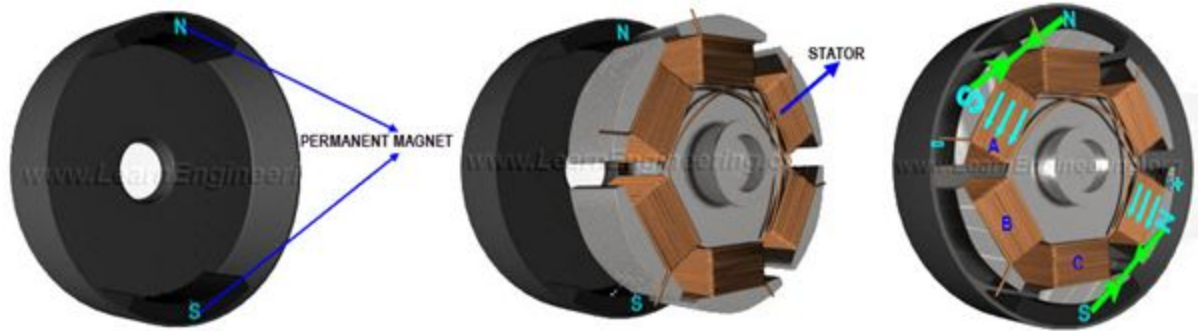
Figure 7: Brushless DC Motor Diagram [13]
